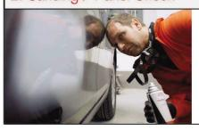
Spray the panel after the sanding process to check repaired surfaces on irregularities.
